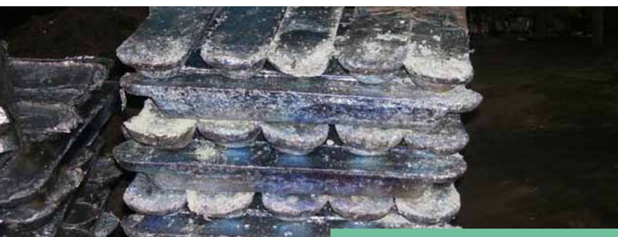
Lead bars at a ULAB recycling site
