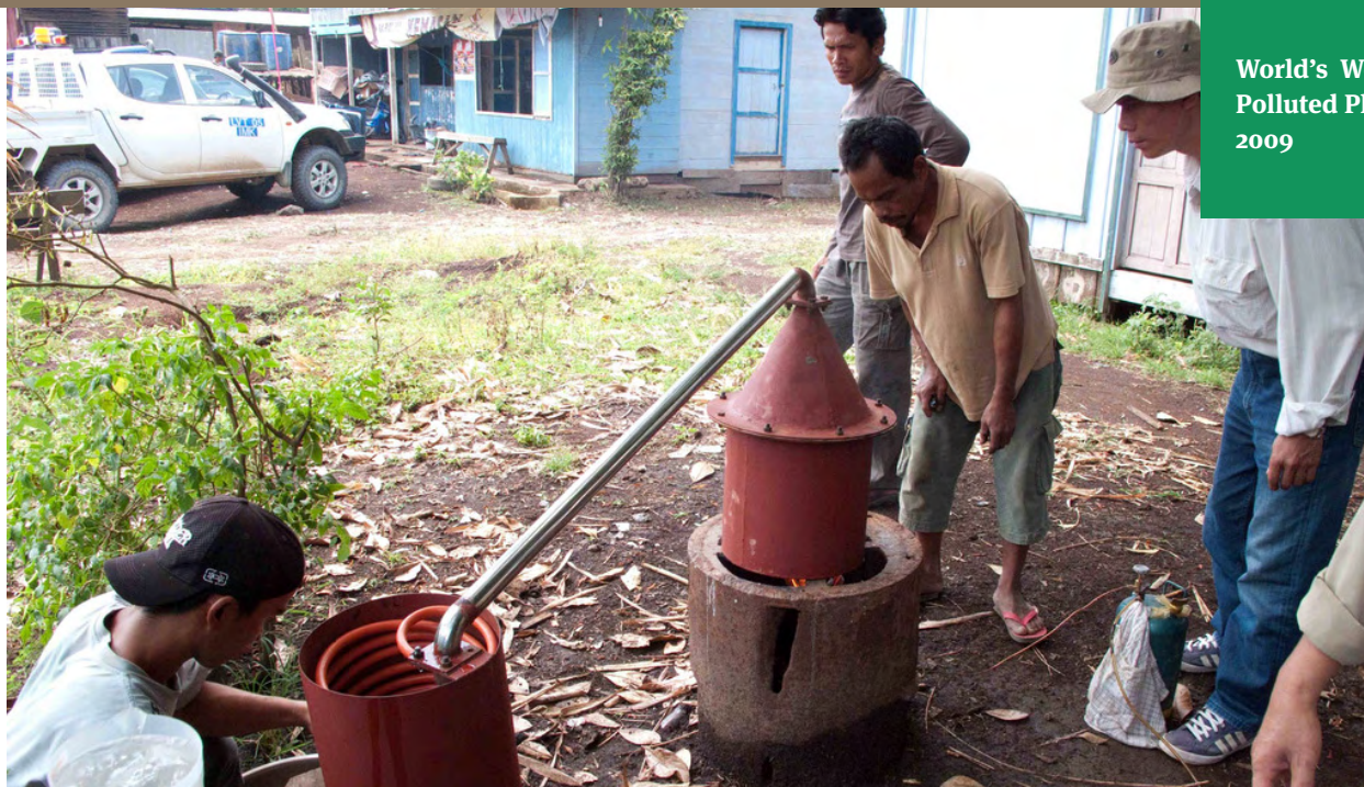
Kalimantan's gold mining community is involved in ongoing developing of retort technology. Credit: Yayasan Tambuhak Sinta
